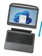
2 Fold the kickstand and keyboard toward the DT323RP tablet for portability and as a protective cover to shield the screen.
